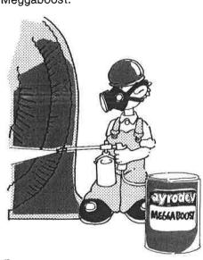
**5.** Concentrate on the areas showing most insulation meter reaction. As each section becomes stable, move to another area. Where possible, rotate the workpiece from time to time.
